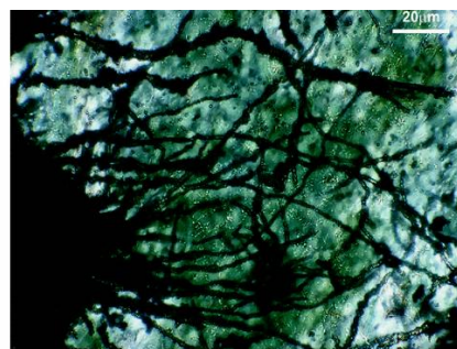
Fig. B63 Thin section image of micro-tubular structures within the Euro Basalt (Photograph courtesy of Nicola McLoughlin)
